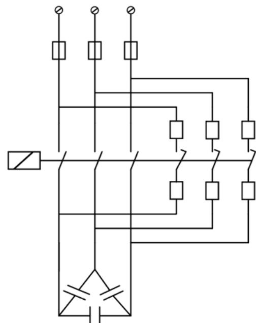
Contactor with pre-charge resistors
