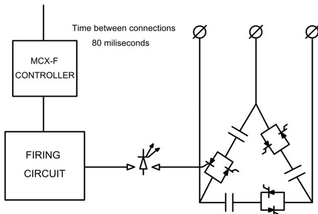
Figure 1: Automatic capacitor bank with static control
