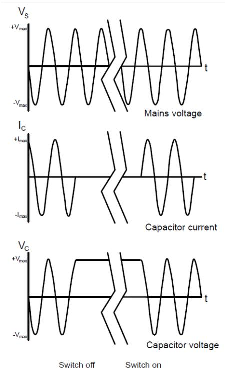
Figure 3: Switching on/off in a capacitor bank with static control
