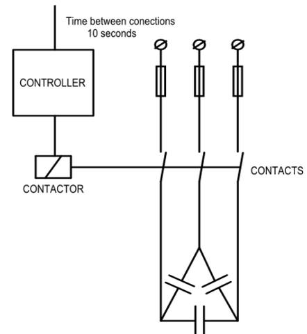
Figure 2: Automatic capacitor bank with contactors
