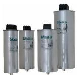
The installation of the capacitors should consider the rules and recommendations of **IEC 60831-1/2** Standard. The capacitors are for **indoor** installation away from heat sources and in well-ventilated places. There shall be a minimum distance of **20 mm** between capacitors. Check that the voltage and frequency given on the capacitor name plate are appropriate for the mains where it is to be installed.
